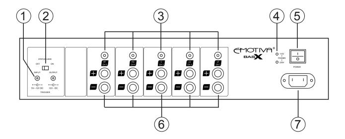
Note: The BASX A-150, BASX A-300, BASX A-500, and BASX A-700 have identical features and controls, and differ only in the power and number of amplifier channels they provide. The BASX A-500 is shown here for illustration.
