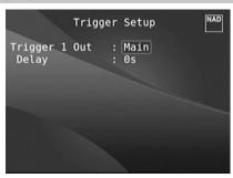
The T 758 features a configurable +12V TRIGGER OUT that can be used to activate a component or system it is fed into. It is used to turn on/off other compliant devices.
