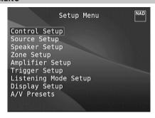
The Setup Menu allows one to customize the operation of the T758 to the ancillary equipment used in one's specific AV system. Unless your system exactly matches the factory defaults as shown in the accompanying Quick Start Guide, you will need to use the setup menu to configure the inputs of the T758.
